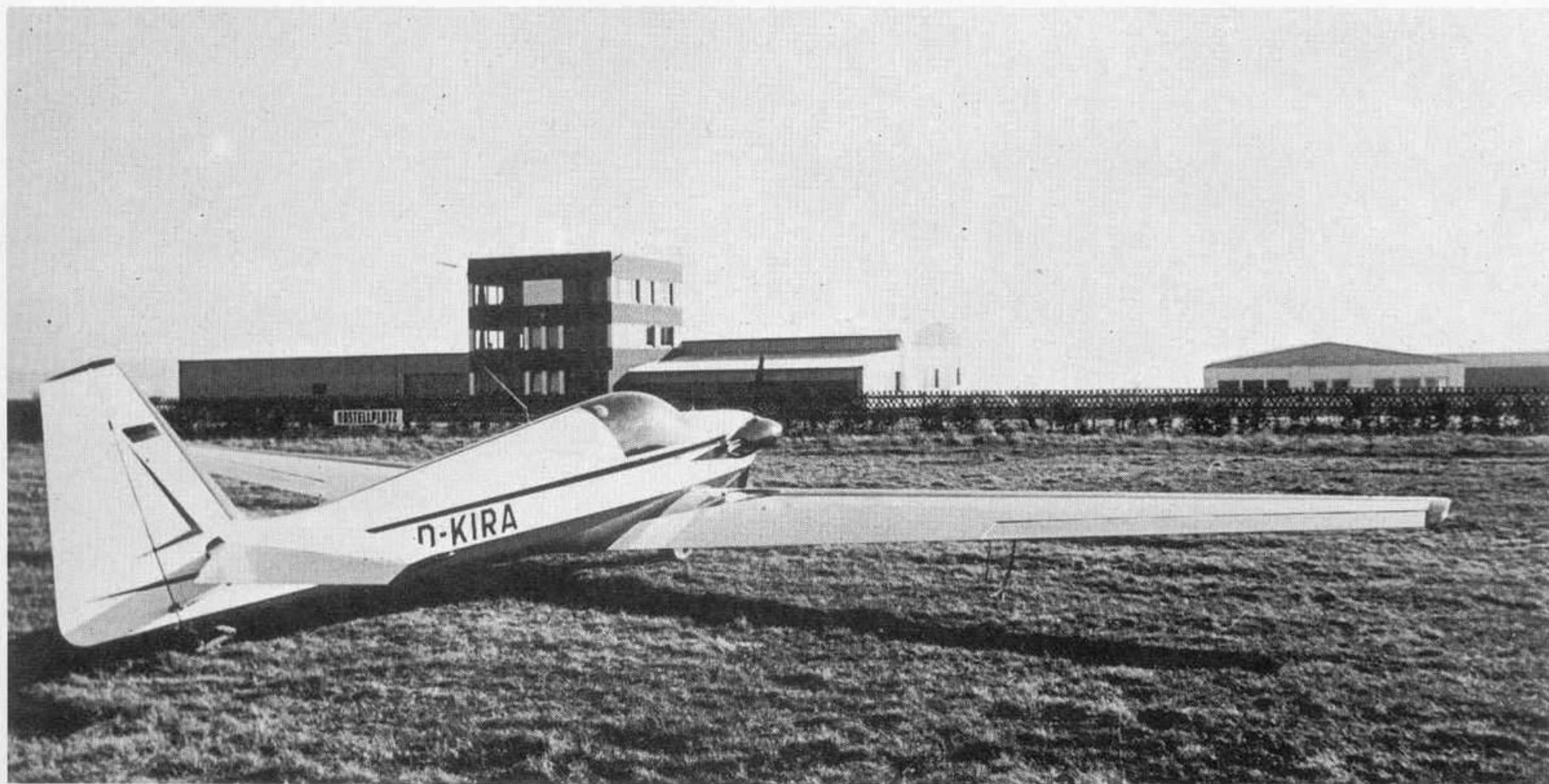
The unconventional bicycle landing gear gives the R.F. 4 the appearance of a U2 in miniature.
