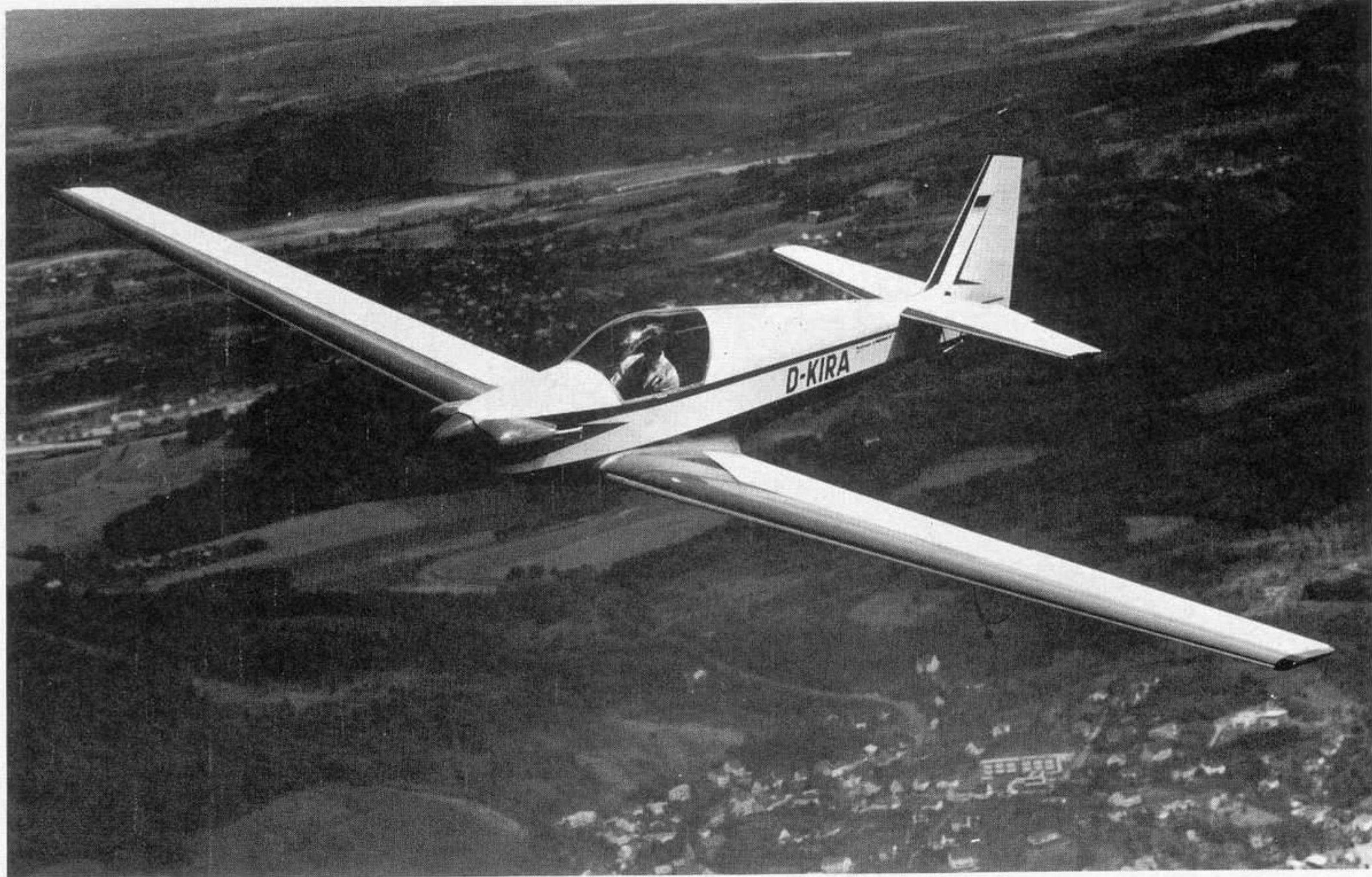
The VW powered RF4 single seater combines aerodynamic efficiency and aerobatic performance deliberately designed into it.
