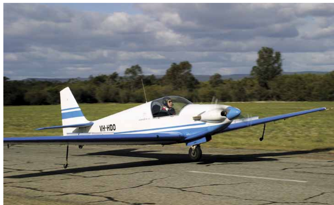
ABOVE: the RF4D's monowheel handling is not difficult, but different and having some taildragger experience helps one master it
