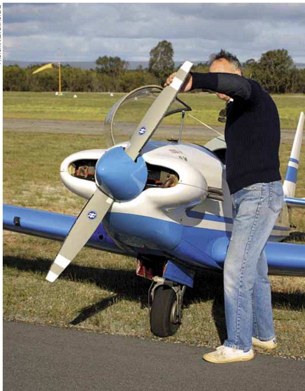
ABOVE: it may look unconventional but this is the easiest and safest way to hand-swing the prop to start the Fournier's little VW engine
