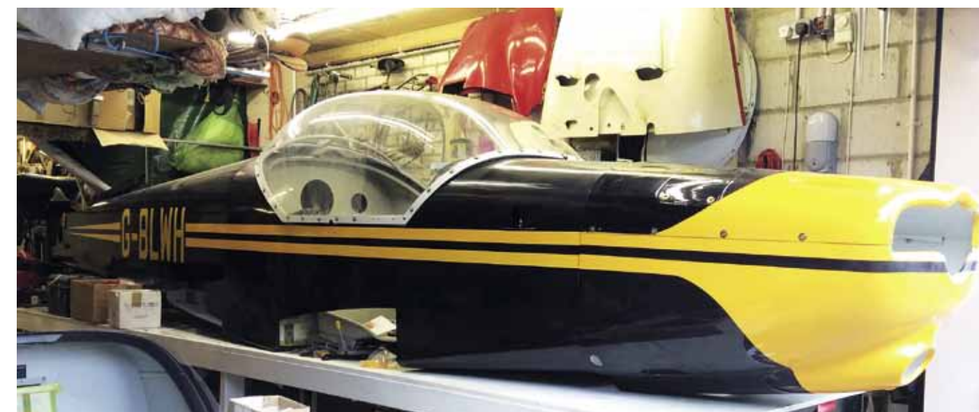
Room for the RF6B fuselage (just) in Bob's home garage workshop. Job One was refitting and adjusting the 'up and over' canopy mechanism
