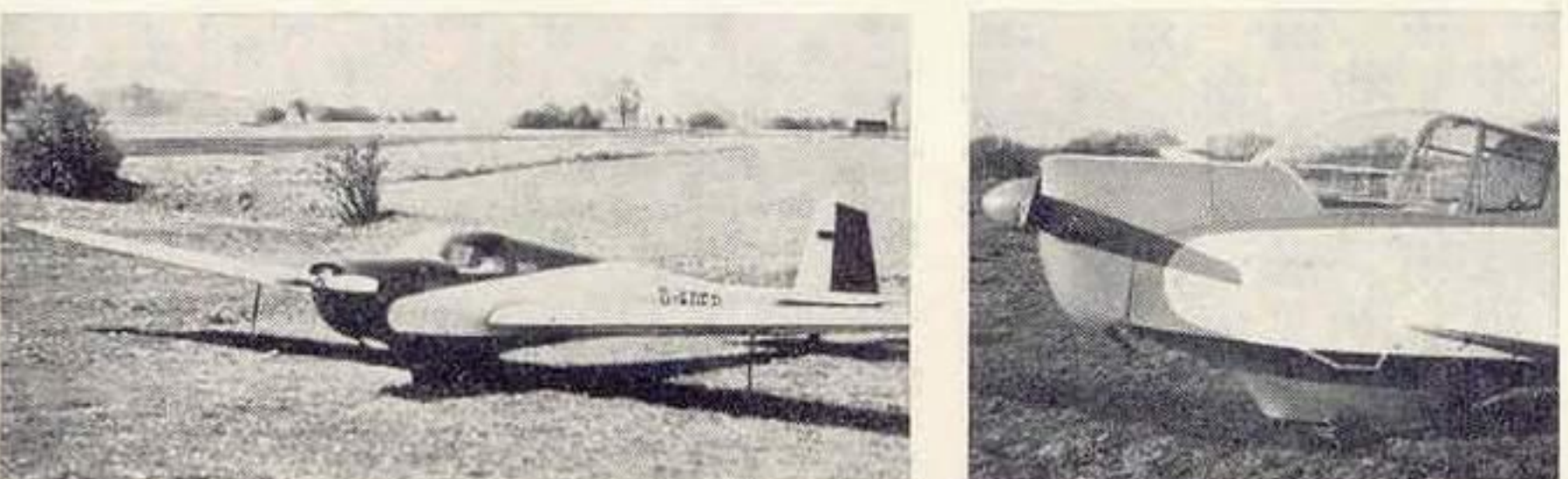
The new two-place Scheibe SF-25B has a 45-hp Stamo 1400-cc engine that uses Volkswagen and Porsche parts.
