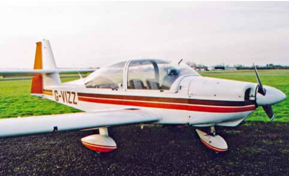
Fitted with a big bubble canopy, cruciform tail and 180hp engine, the RS180 was a development of the RF6C three/four seater that proved equally uncompetitive with American all-metal designs
