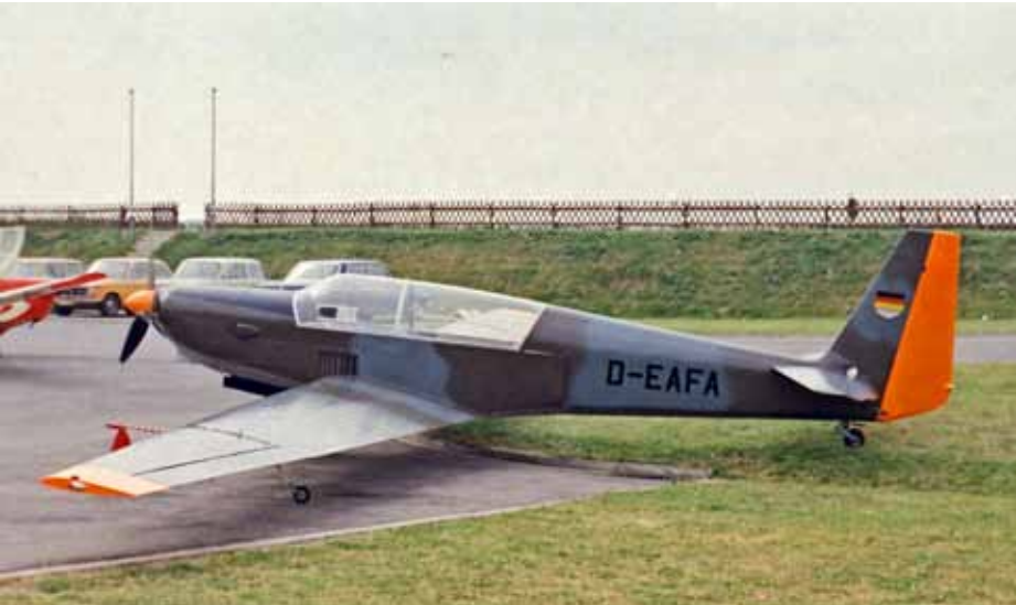
Fitted with a Lycoming O-235, broad-chord three-bladed Hoffmann propeller, extensive exhaust silencing and infra-red shielding, the Sportavia S5 was a 'stealth' machine intended for military use
