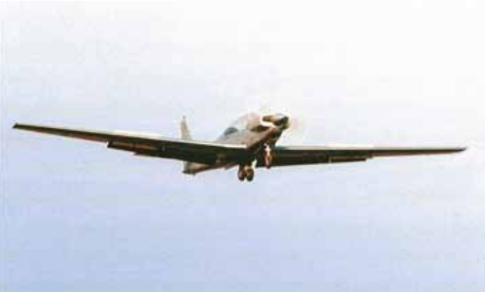
Only one prototype of the all-metal bicycle undercarriage RF8 military trainer was built. The project died for lack of funding
