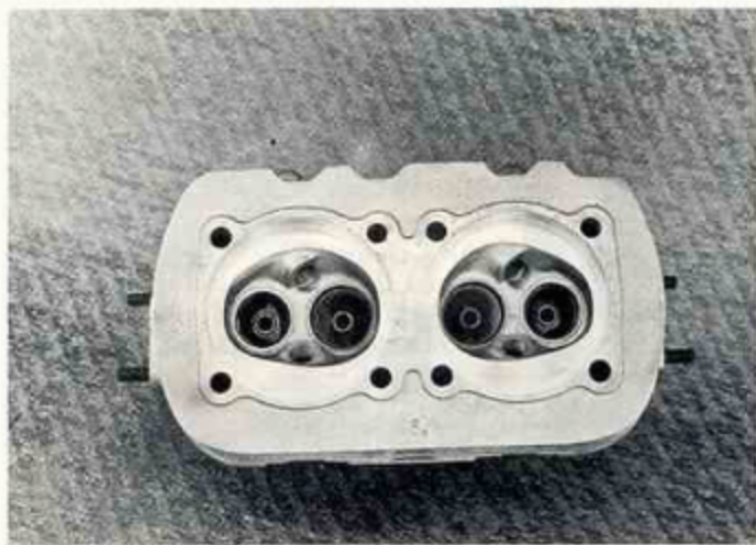
Close up of the combustion chamber on a Limbach dual ignition head. The additional material cast into the head which will provide sufficient threads for the second spark plug can be clearly seen.
