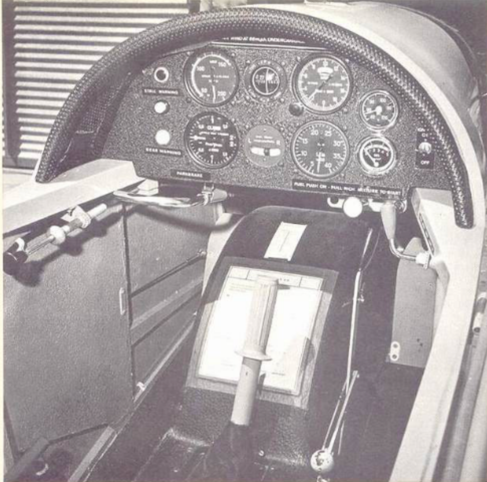
Cockpit and instrument panel of the RF4D. Knob on the floor is the gear lock. The author found labels on fuel and choke confusing (choke knob is concealed by the lever handle on the right side). Both should be forward for takeoff and flight.
